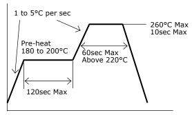
• Recommended Hand Soldering Condition
